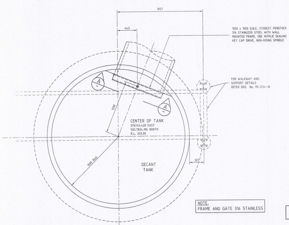
PLAN OF PRIMARY SPILLWAY INLET AND PENSTOCK
