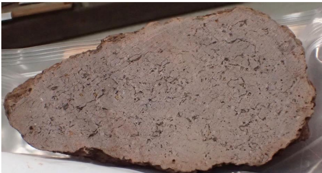
Fig. 20. G408836. Cut surface showing a spotty agglutinate texture in basalt, composed of small welded lapilli. FOV ~150mm
