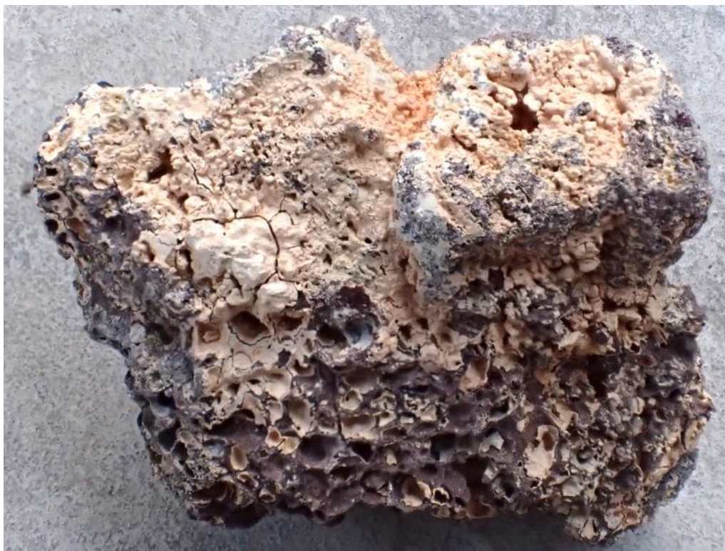
Fig. 4. C112293. Scoriaceous basaltic breccia, showing abundant white clay infilling vesicles. FOV ~100mm
