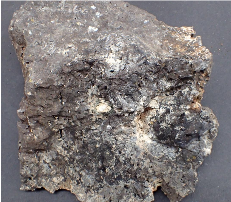
Fig. 9. C112296. Vesicular basalt, showing white minerals filling vesicles. FOV ~120mm
