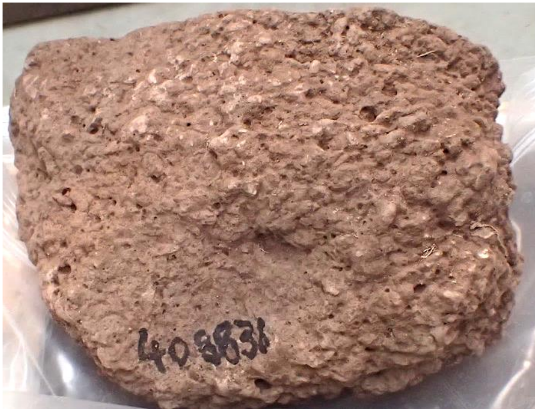
Fig. 19. G408836. Agglutinate texture in basalt, showing small welded lapilli. FOV ~120mm
