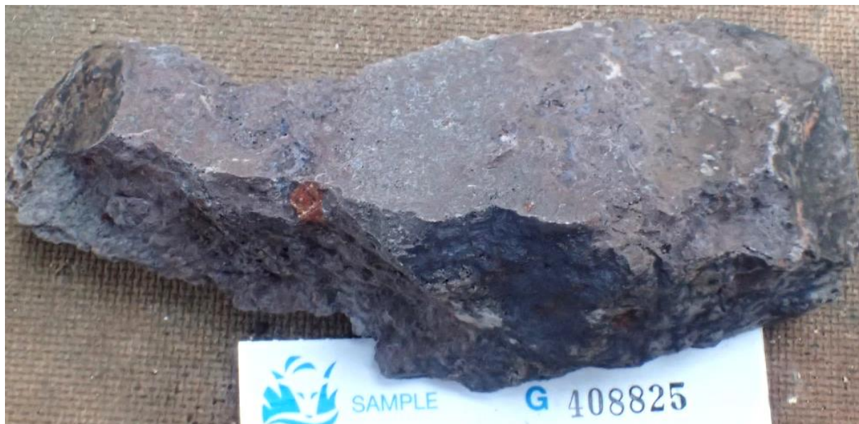
Fig. 16. G408825. Non-vesicular basaltic rock which appears to have been silicified. FOV ~120mm
