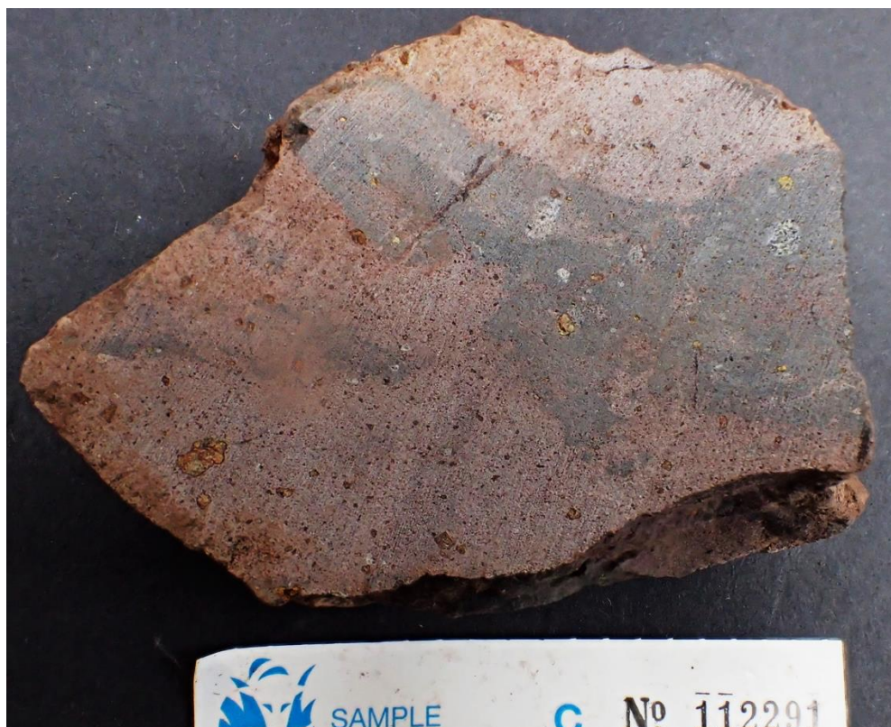
Fig. 2. C112291. Autoclastic, scoriaceous basaltic breccia, cut face, showing a variably scoriaceous texture plus small xenoliths and phenocrysts. FOV ~110mm
