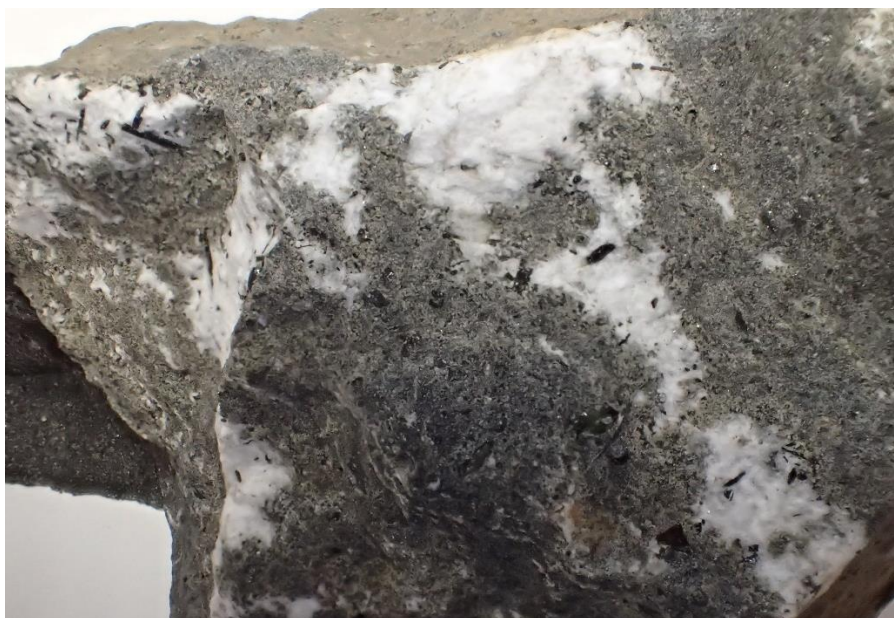
Fig. 2: G407355. White zeolite veins, with black pyroxenes, in basalt. FOV: about 45 mm.
