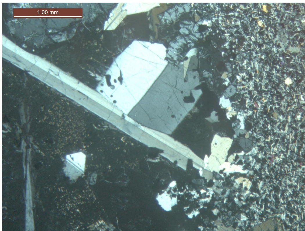
Fig. 19. Sample G408090b, Polarised light, crossed polars, showing a glassy segregation in basalt, with speckled black sideromelane, coarse, colourless, blocky crystals of nepheline (top), twinned prismatic clinopyroxenes and prismatic apatite (lower left). FOV 5mm.
