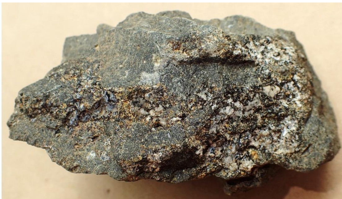
Fig. 3: Sample G408090a, showing cavities containing zeolites, nepheline, pyroxene and other minerals, in cavities in basalt. FOV: about 60 mm.
