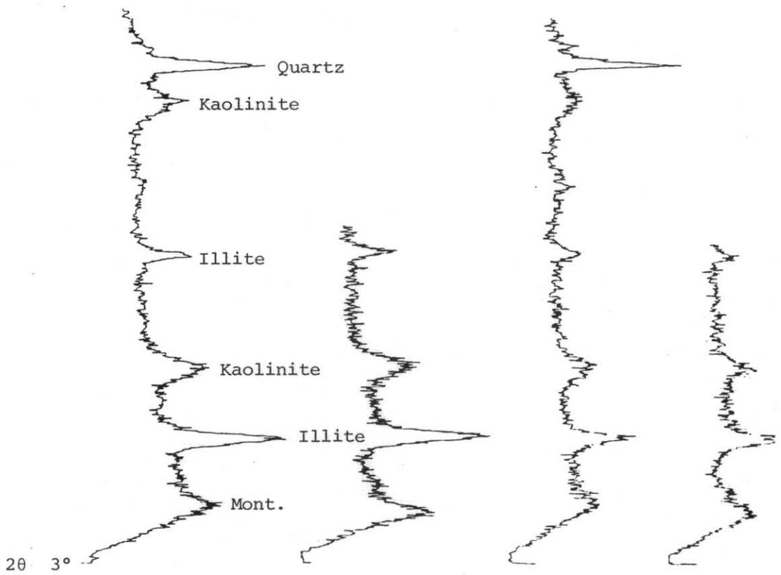
Figure 1. Diffractograms of (a) Core 3, (b) Core 3 - glycolated, (c) Core 4, (d) Core 4 - glycolated. Mont. = Montmorillonite.
