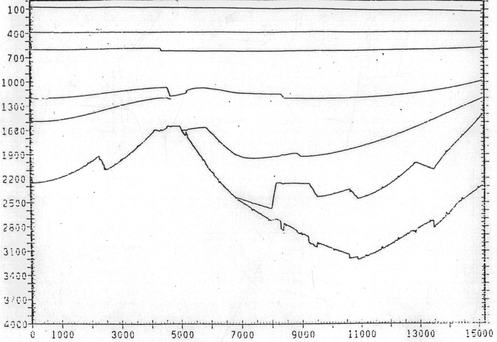
FIGURE 6.9 IMAGE RAYS FOR SMOOTHED VELOCITY FUNCTION
