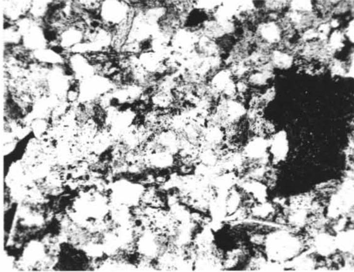
Narimba-1 9278' depth L-M Eocene. Siderite nodule in very fine lithic sandstone (x 92, plane-polarised light).
