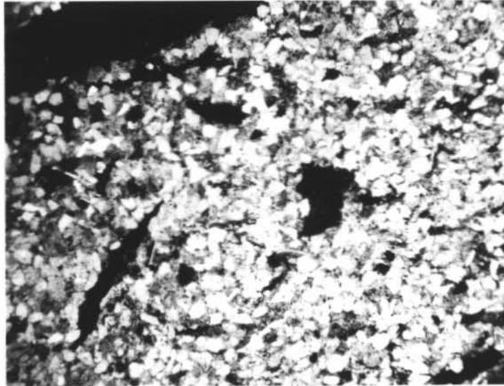
Narimba-1 9278' depth, L-M Eocene. Very fine lithic sandstone with carbonaceous stringers (top left) and siderite nodules (centre). Porosity 13.1%, permeability less than 0.1 mD (x 37, plane-polarised light).
