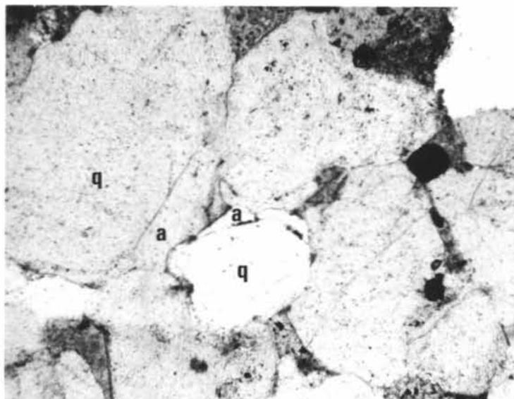
Narimba-1 9750' depth, L-M Eocene. Coarse sandstone; authigenic quartz overgrowths (a) on detrital quartz (q) grains (x 92, plane-polarised light).
