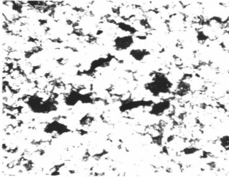
Narimba-1 9548' depth, L-M Eocene. Fine to medium sandstone composed of quartz, feldspar and lithoclasts; black angular areas in lower left are voids. Porosity 19.2%, permeability 0.95 mD (x 37, plane-polarised light).
