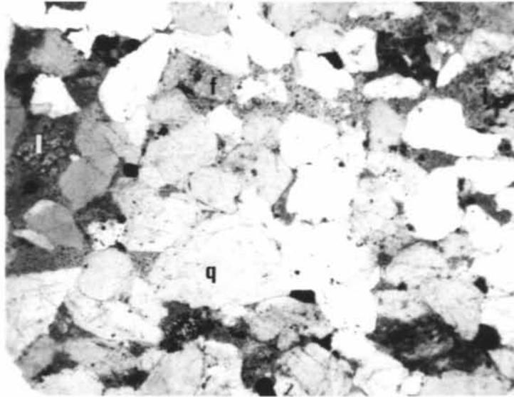
Narimba-1 9750' depth, L-M Eocene. Coarse sandstone composed of quartz (q), lithoclasts (l) and feldspar (f); cemented by authigenic quartz overgrowths. Porosity 19.4%, permeability 54 mD (x 37, plane-polarised light).
