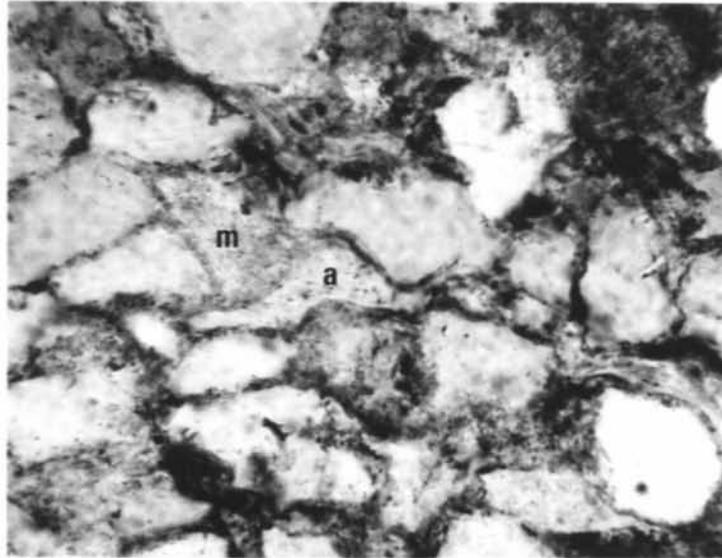
Narimba-1 9298' depth, L-M Eocene. Very fine micaceous sandstone; muscovite (m) slightly contorted and partly enclosed by authigenic quartz (a). Porosity 12.3%, permeability less than 0.1 mD (x 230, plane-polarised light).
