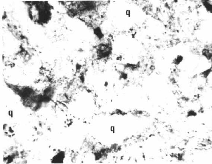
Narimba-1 9302' depth, L-M Eocene. Very fine micaceous sandstone, mica distributed between quartz grains. Some quartz grains (q) with authigenic overgrowths. Porosity 11.4%, permeability less than 0.1 mD (x 230, plane-polarised light).
