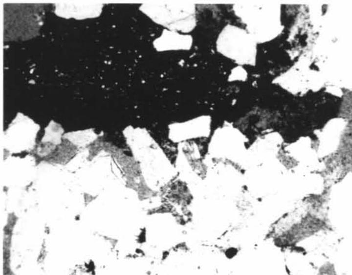
Narimba-1 9750' depth, L-M Eocene. Clay drape (black) in coarse quartz sandstone (x 37, plane-polarised light).
