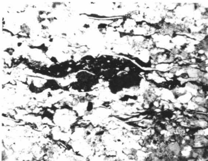
Narimba-1 9544' depth, L-M Eocene. Siderite nodules (black, centre) in very fine, micaceous sideritic sandstone. Porosity 16.7%, permeability 2.2 mD (x 37, plane-polarised light).
