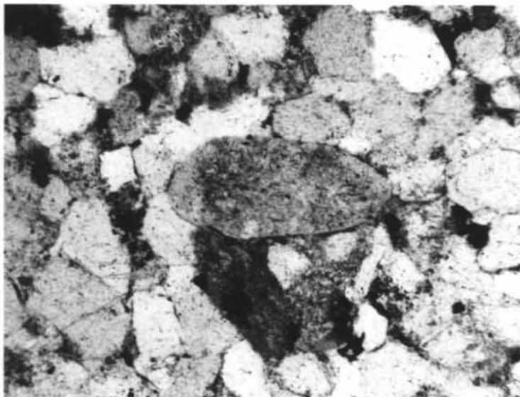
Narimba-1 9548' depth, L-M Eocene. Chert grain surrounded by quartz grains; advanced authigenic quartz overgrowths on quartz grains, but no overgrowths on the chert grain (x 92, plane-polarised light).
