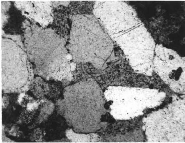
Narimba-1 9750', L-M Eocene. Large kaolinite patch (grey, centre right) is probably kaolinised feldspar or volcanoclast (x 92, plane-polarised light).
