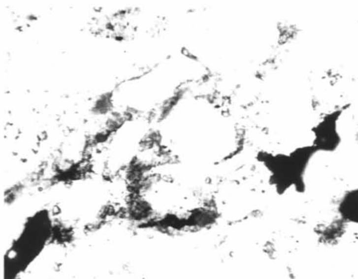
Narimba-1 9278' depth, L-M Eocene. Quartz grain (centre white) partly covered by siderite crystals (x 230, plane-polarised light).
