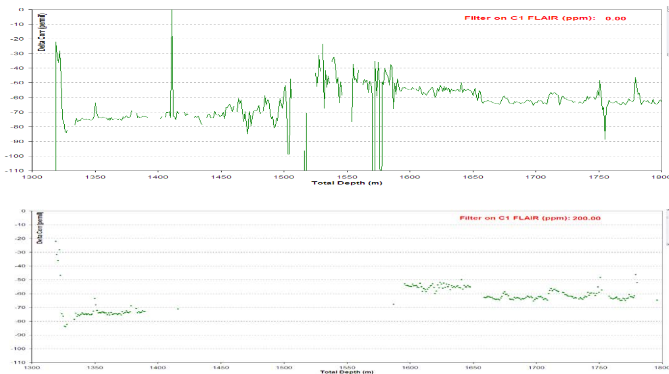
Fig. 5: \delta^{13}\text{C} without any filter (top part), and filtered with a limit of 200 ppm on C1 (lower part). This limit is determined from the logged section 1400 mMD to 1600 mMD, where the gas level in FLAIR drops.
