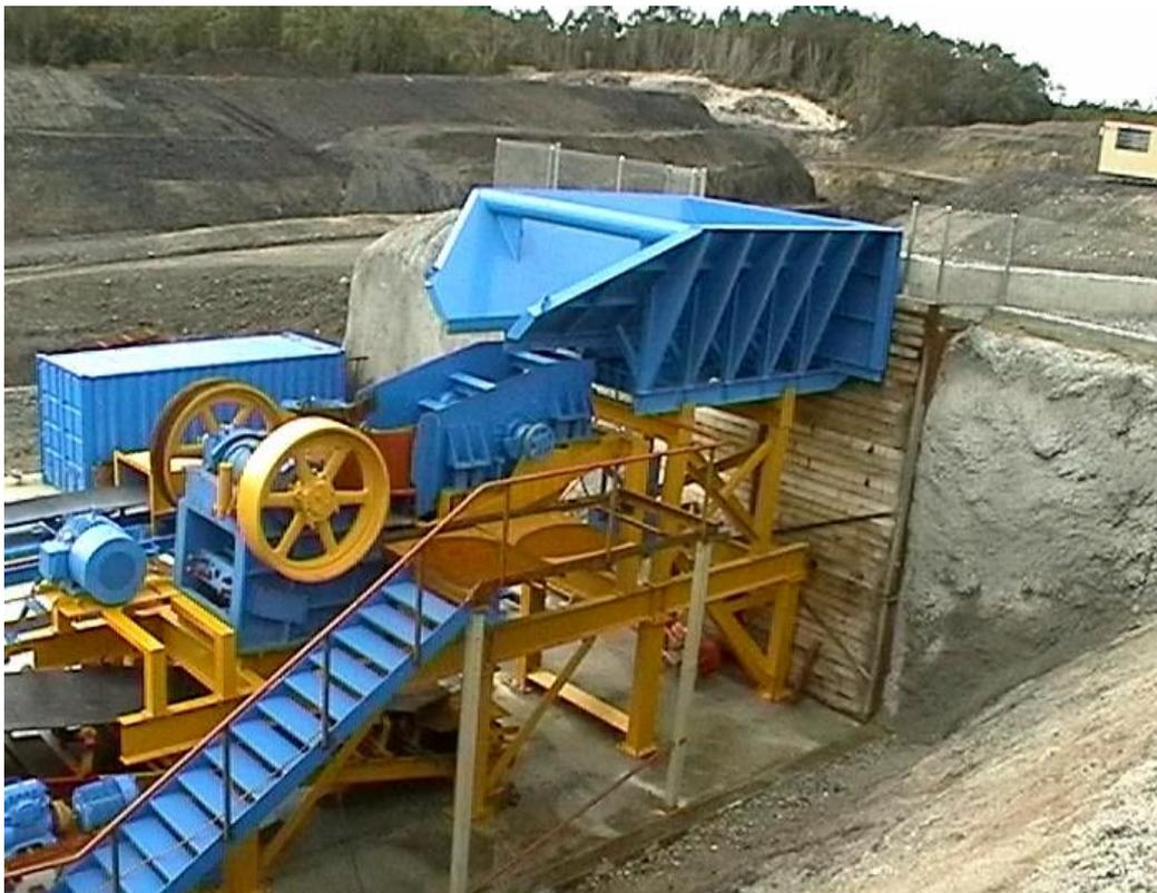
**Figure 8.** Coarse Ore Bin & Primary Jaw Crusher
