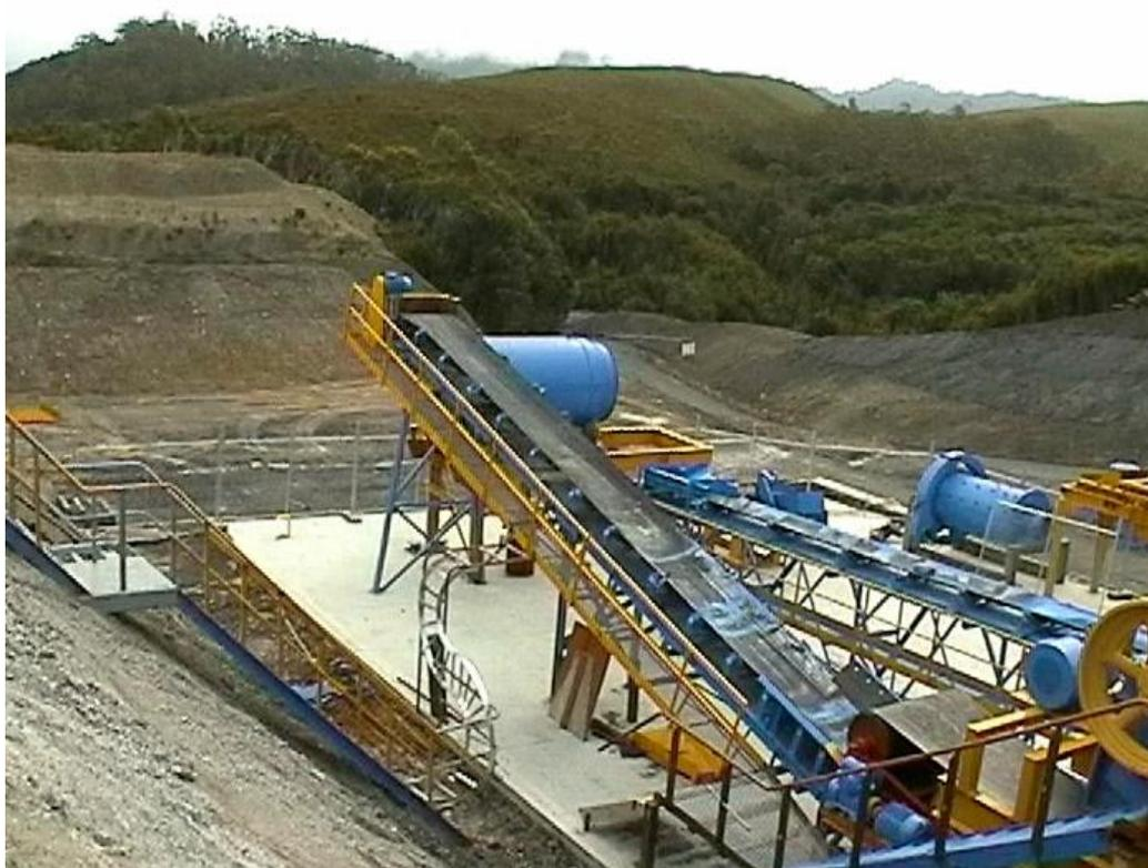
**Figure 6.** Primary Jaw Crusher (right), Conveyor (centre) that feeds into Trommel.
