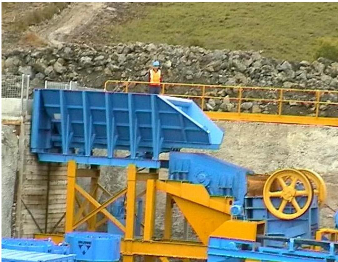
**Figure 9.** Coarse ore bin feeding into Primary jaw crusher with 10,000 tonne high grade ore stock pile in background (20% zinc, 10% lead).
