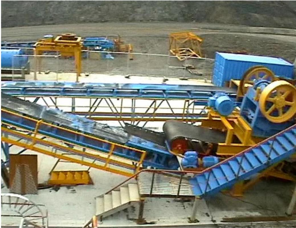
**Figure 7.** Primary Jaw Crusher (right), weightometer, conveyor.
