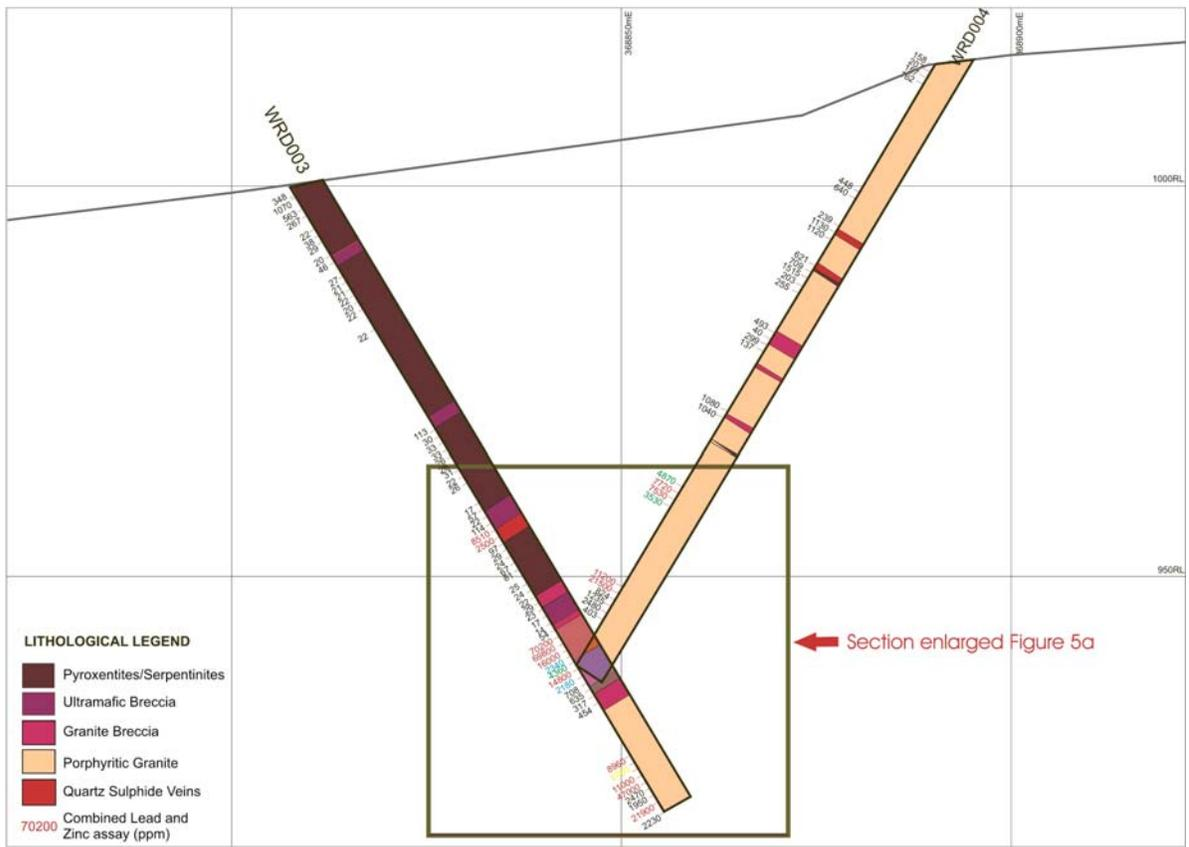
**Figure 6a.** Enlargement of drilling Cross section, of holes WRD03, WRD04, showing combined lead and zinc assays (%)
