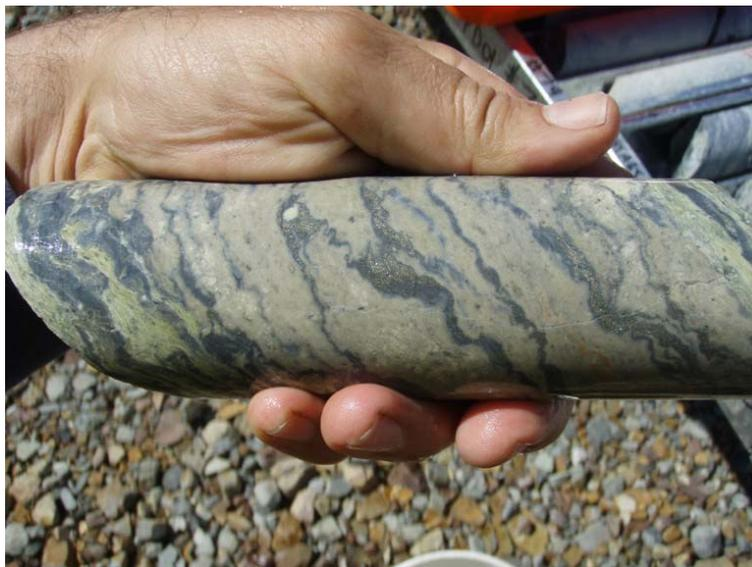
**Figure 8. Example of sulphide stingers in pumice breccia from drillhole PD01.**
