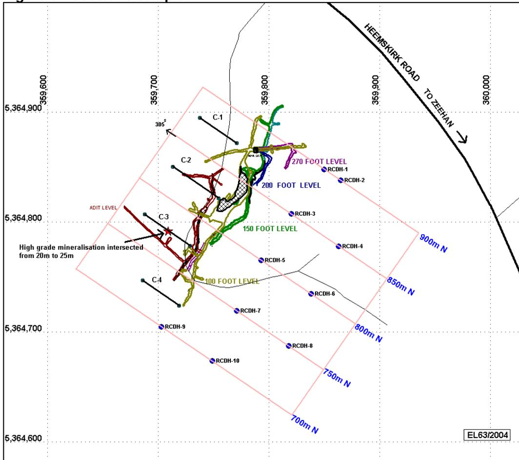
Results were received for the costean sampling with the best intercepts being 7m at 4.7% Pb, 2.8% Zn and 650 g/t Ag. The only other significant intersection was 3m at 1.9% Pb 3.8% Zn and 35 g/t Ag
