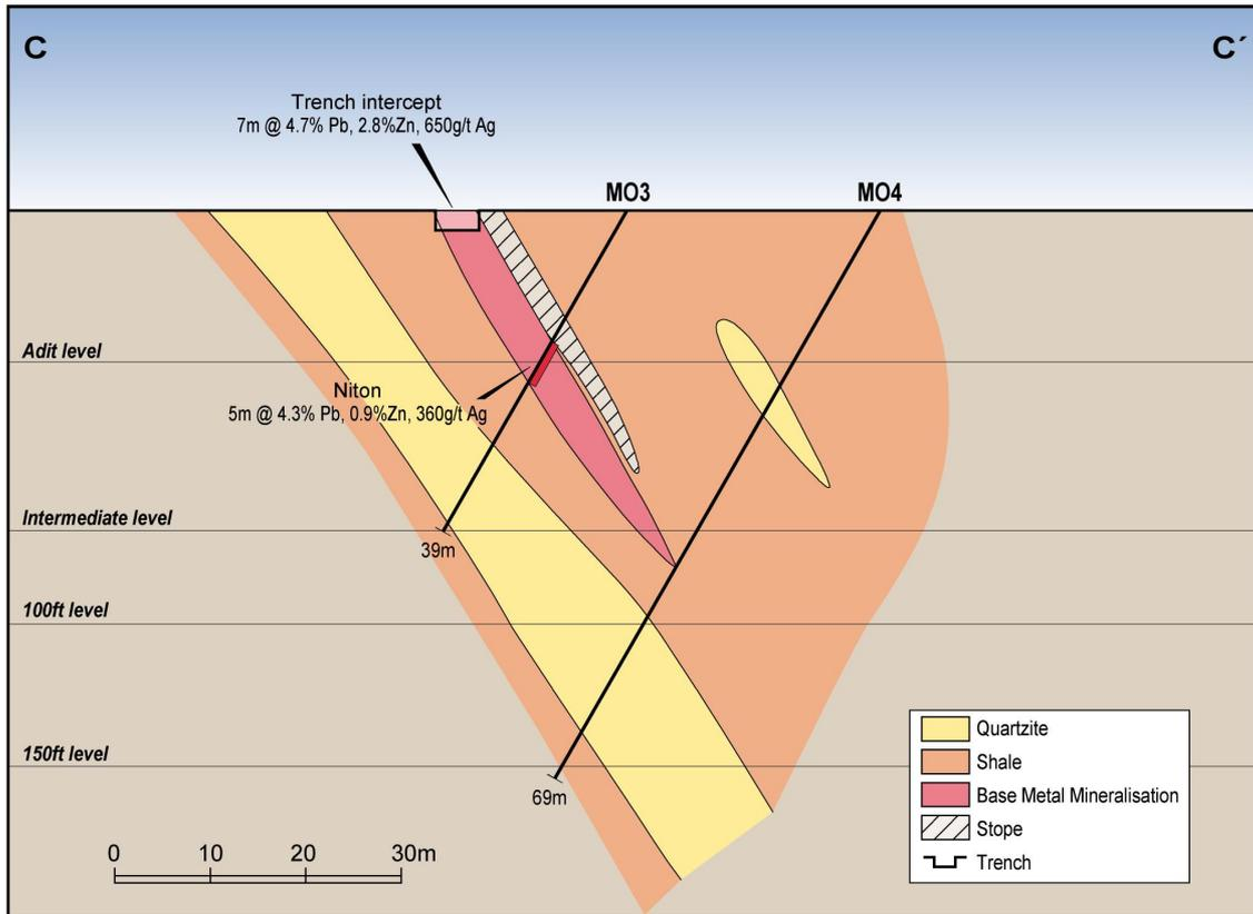
**Figure 7. The Sections drawn in MapInfo including Shear Zone, Stope and pierce points of each RC drill hole.**
