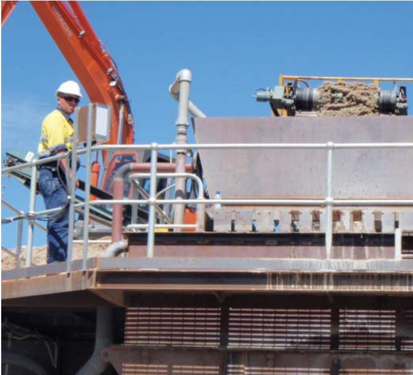
**Photo;** Shows dry feed feeding into the bin with water manifolds aiming at the drop point to slurry the feed as it passes the top sizing grizzly. The excavator in the background is feeding the bin as an interim measure to manage the top size limit on feed going into the main slurry feed pump.
