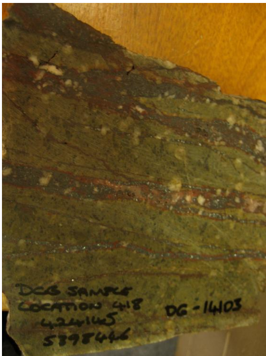
Photo 35. Hematite veining and passive replacement textures in volcanoclastic
