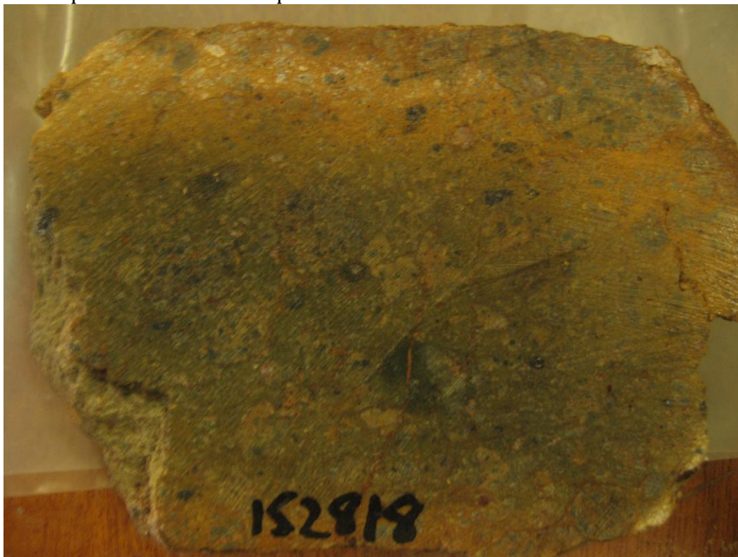
Photo 31. Sample 152818. Feldspar-phyric volcaniclastic, with sericitised feldspars and chlorite altered groundmass.
