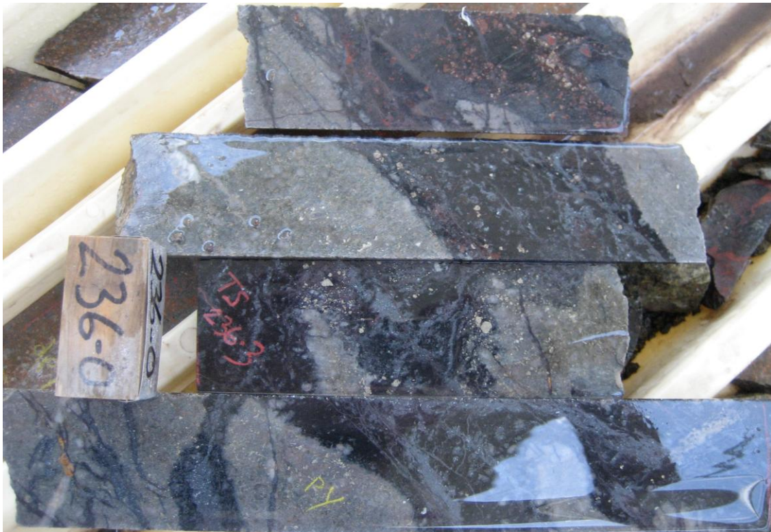
Photo 3. DR1 @ 236 m. Light grey sericite-quartz-pyrite alteration cut by tourmaline and hematite veins.
