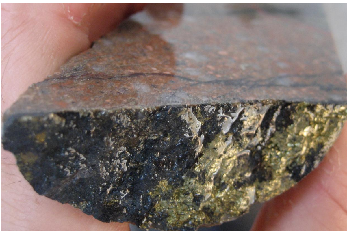
Photo 7. DR1 @ 266m. Hematite + chalcopryite veins, crosscutting K-feldspar zone
