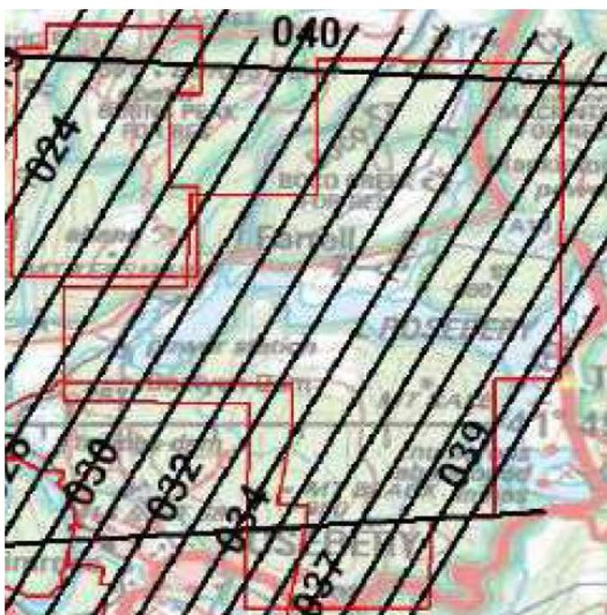
Figure 4: LIDAR Survey flight lines over EL41/2010
