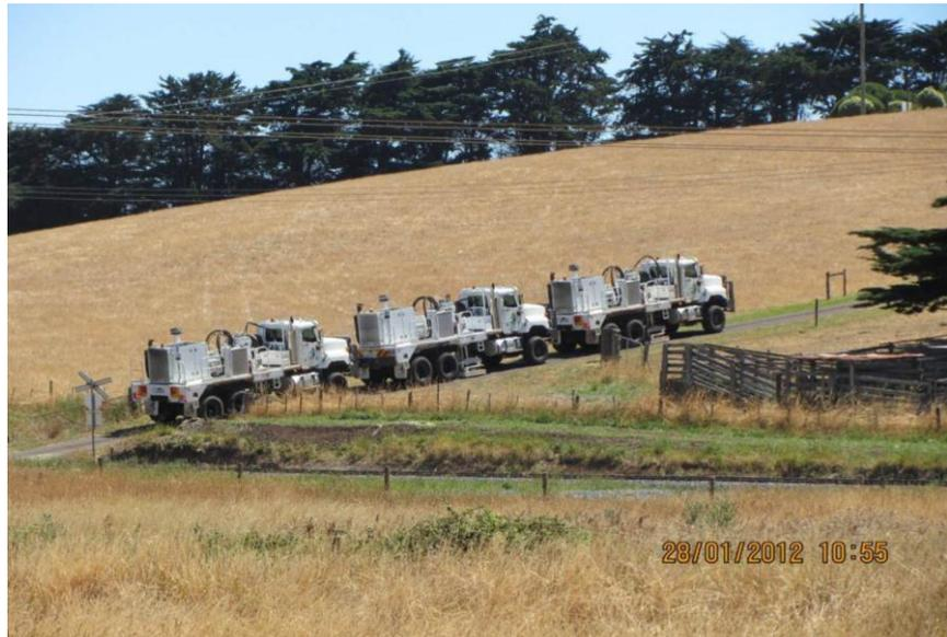
Figure 4: Terrex Seismic Vibro-seis Equipment in SEL 5/2005
