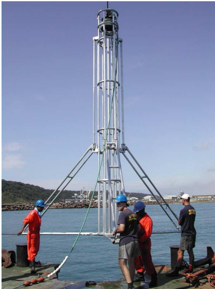
Figure 8: Vibracorer being deployed
