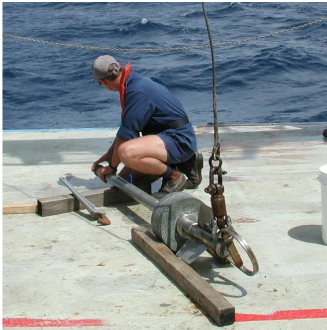
Figure 13: Gravity corer disassembly for core removal
