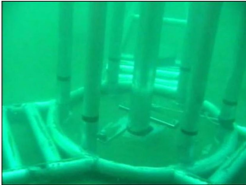
Figure 9: Underwater picture of vibracorer in operation Source: vibracoring video by Marine GeoSolutions
