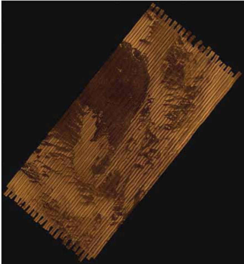
Side-scan sonar mosaic of the seafloor.
