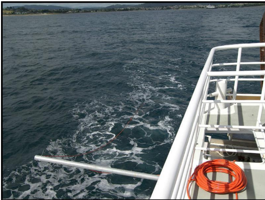
Hydrophone array (orange cable) being towed astern of the vessel.
