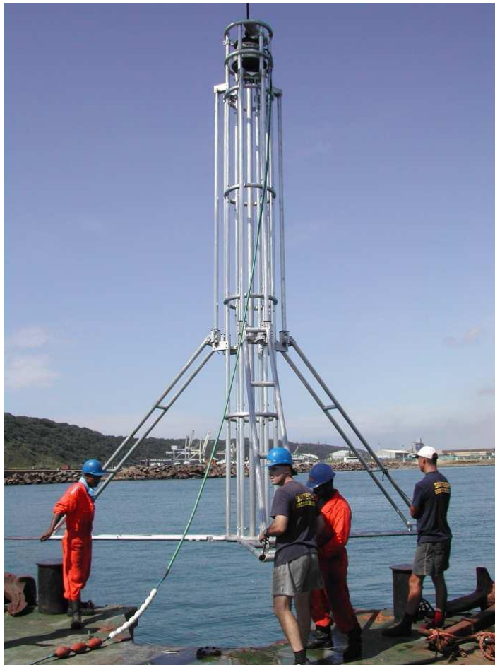
Figure 8: Vibracorer being deployed
