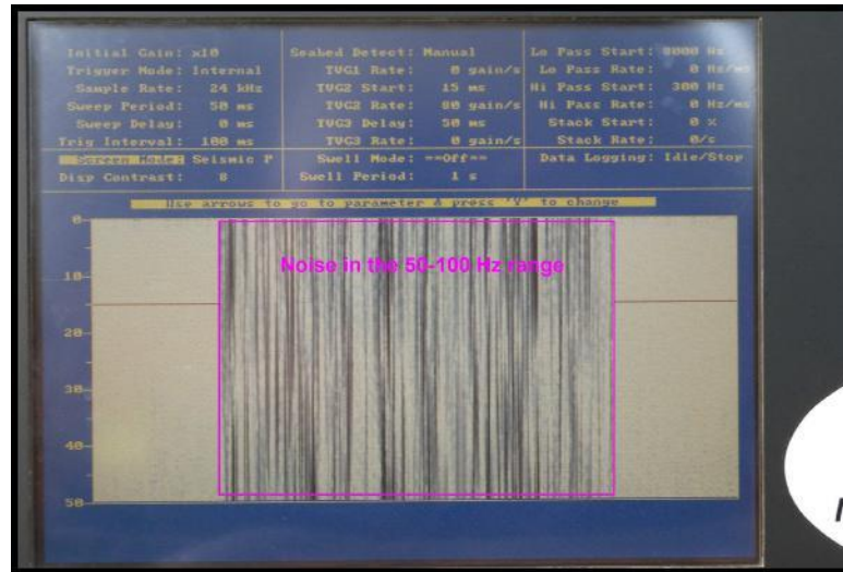
Acquisition system screen capture showing raw (unfiltered), noisy data in the middle of the screen flanked by clean bandpass filtered data on either side.
