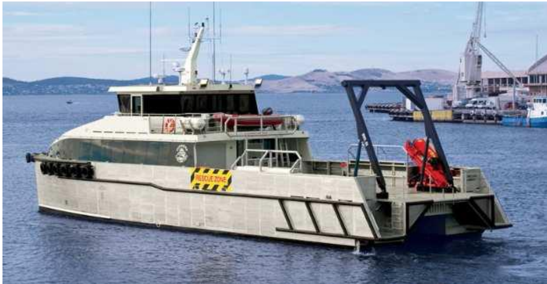
Figure 7: Example of a vessel equipped for vibracoring
