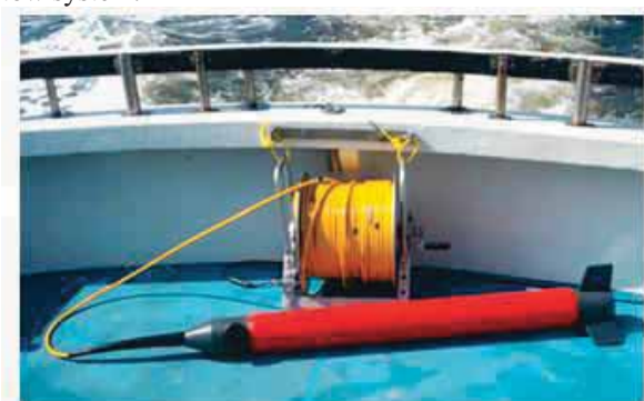
SeaSpy magnetometer and tandem tow system with the side-scan sonar.
