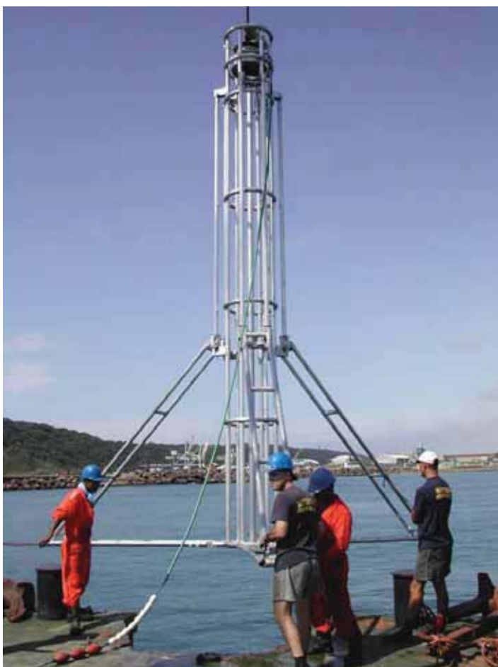
Figure 8: Vibracorer being deployed
