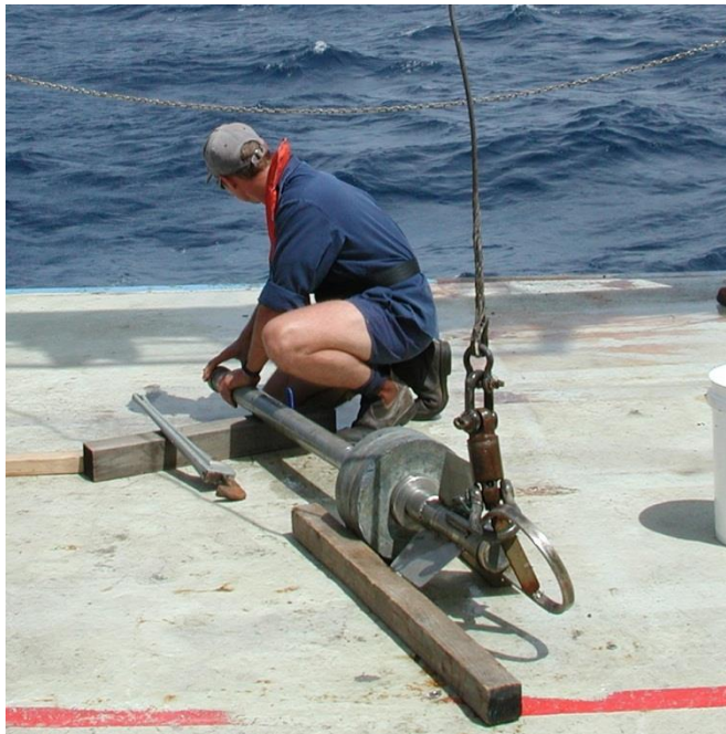
Figure 13: Gravity corer disassembly for core removal
