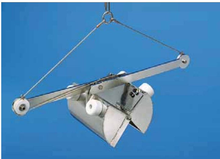
Figure 10: Image of a Shipek Grab sampling bucket
