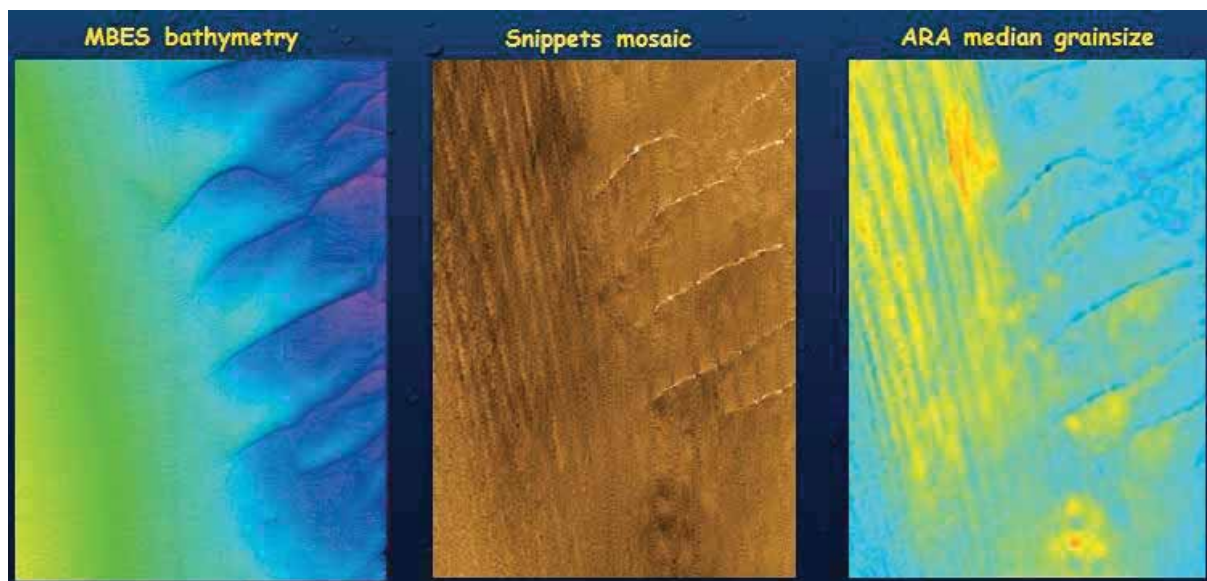
Detailed backscatter processing showing the MBES digital terrain model, backscatter mosaic and backscatter extracted sediment grainsizes.
