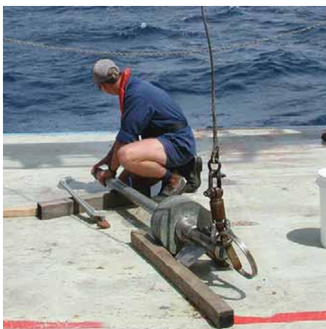
Figure 13: Gravity corer disassembly for core removal
