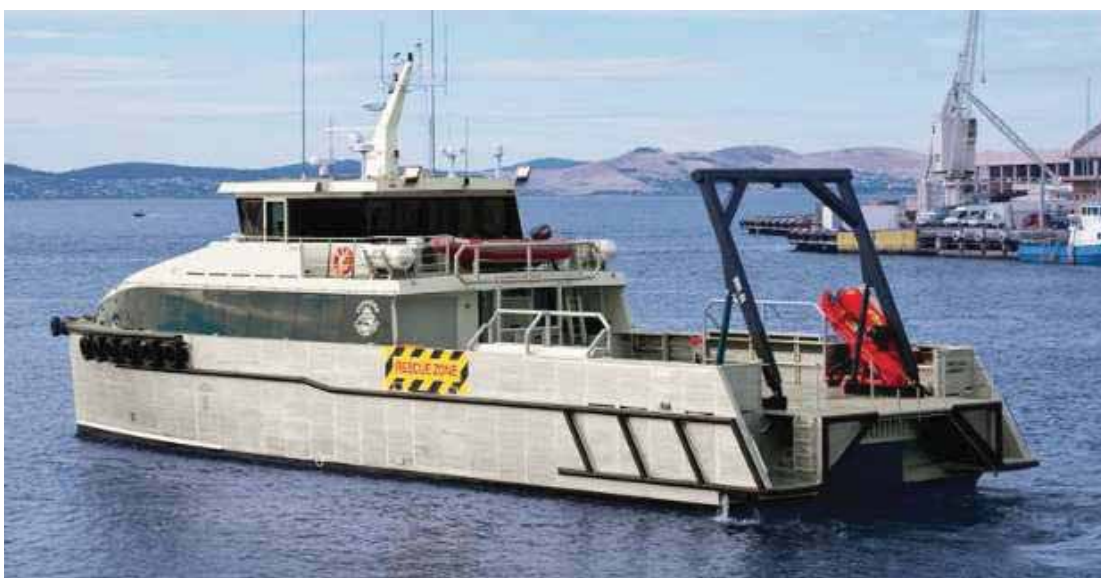
Figure 7: Example of a vessel equipped for vibracoring
