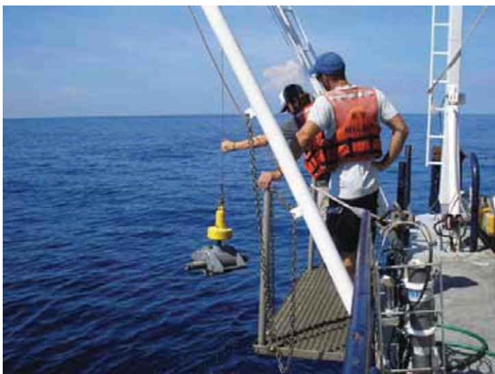
Figure 11: Image of a Shipek Grab being deployed from a vessel
