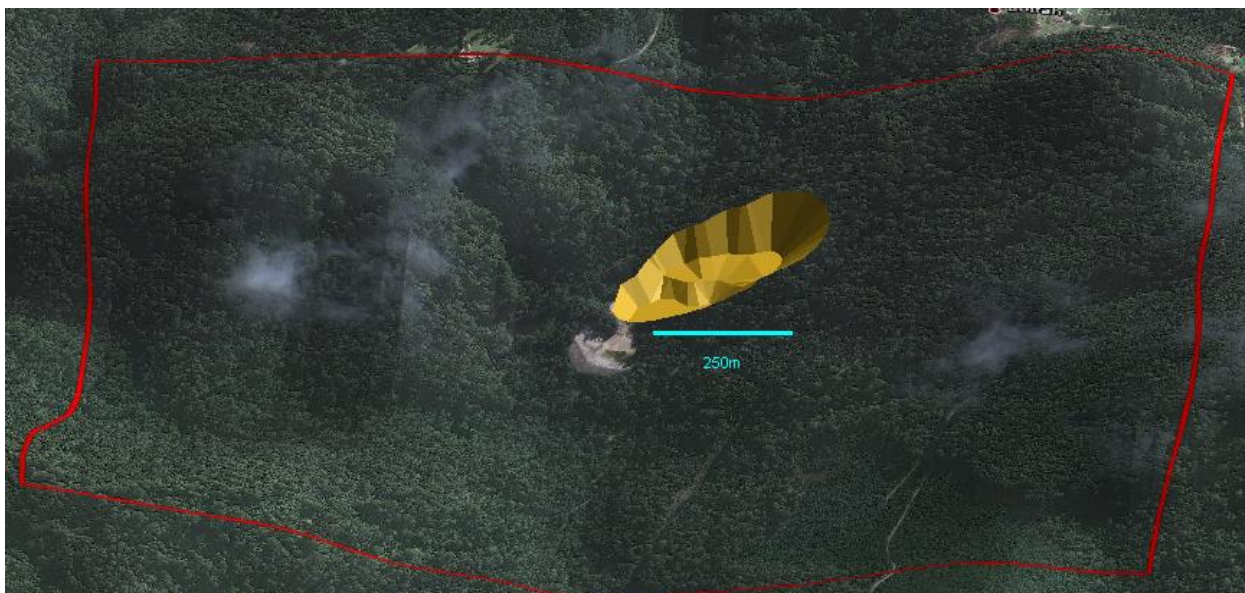
Figure 5: View of conceptual pit based on 3.3Mt of ore and stripping ratio of 2
