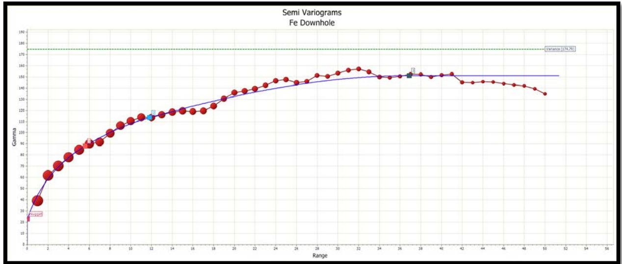
Figure 16 : Downhole experimental Semi Variogram for Fe with model fitted
