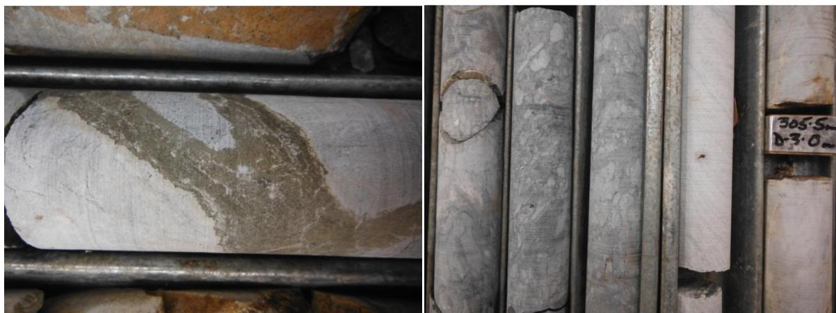
Figure 4: Semi-pervasive green calc-silicate / skarnified zone @387.4m (left) and Oolitic and laminar bedded limestone (right).
