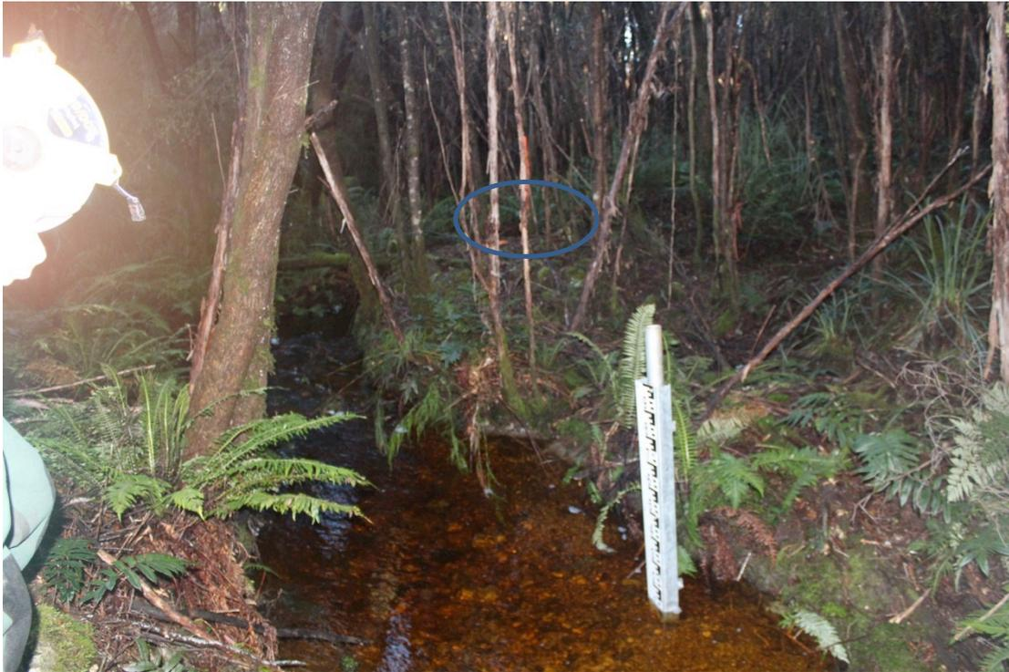
Figure 2 – Webber Creek gauge board with benchmark top middle on earthen mound.
