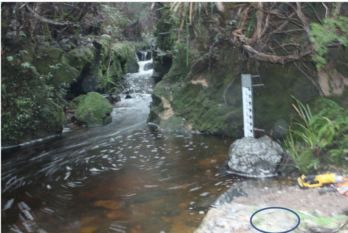
Figure 1 – St Dizier gauge board with benchmark bottom right on rock outcrop.
