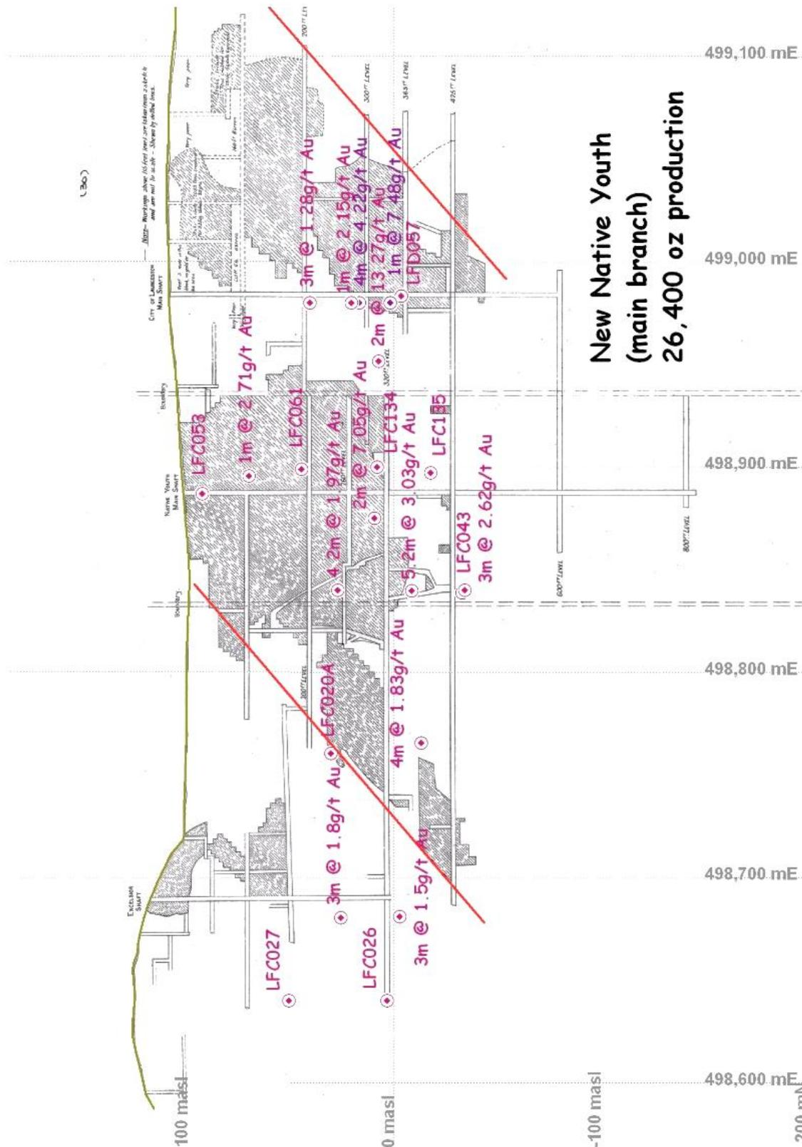
Figure 4.2: New Native Youth mine long section showing main branch stoping - view looking north. Maroon dots are drillhole intersections with the main branch reef, purple dots with a separate minor branch reef. Gold grades are downhole lengths.
