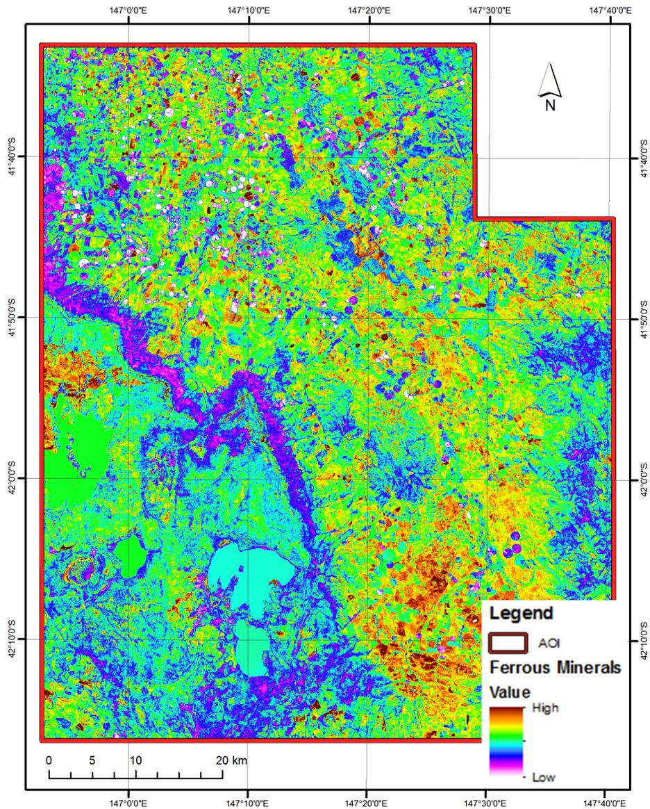
Figure 42: Ferrous minerals concentration; ferrous mineral = Band6/band5.
