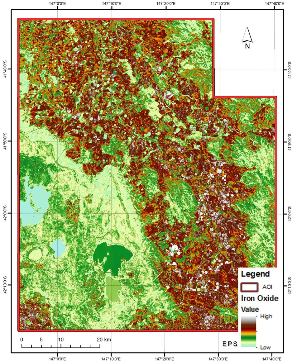
Figure 41: Iron oxide minerals concentration; iron oxide=Band4/band2.
