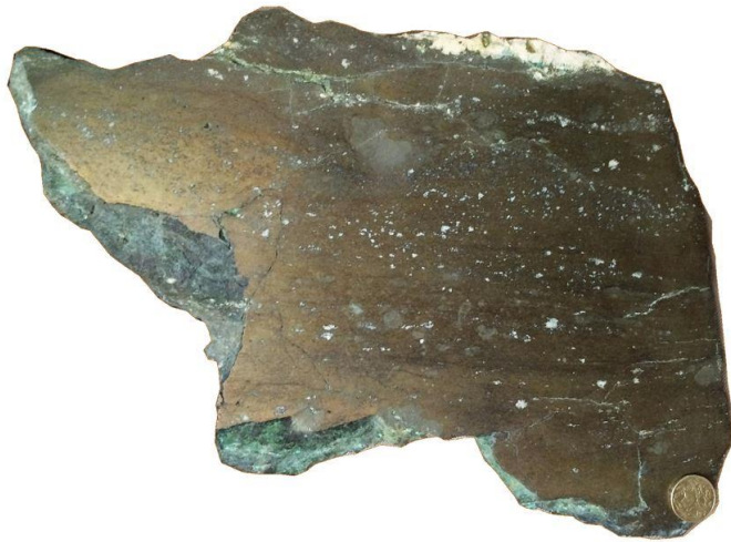
figure 4.2: Massive chalcopyrite from the high grade shoot at Murrays Reward (M. Laan) – note coin for scale.
