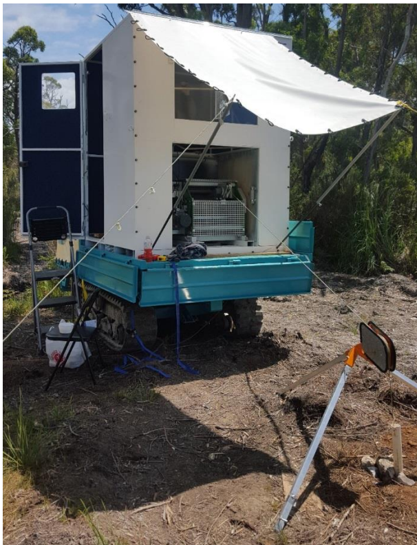
figure 5.3: DigiAtlantis EM system surveying hole at Balfour
