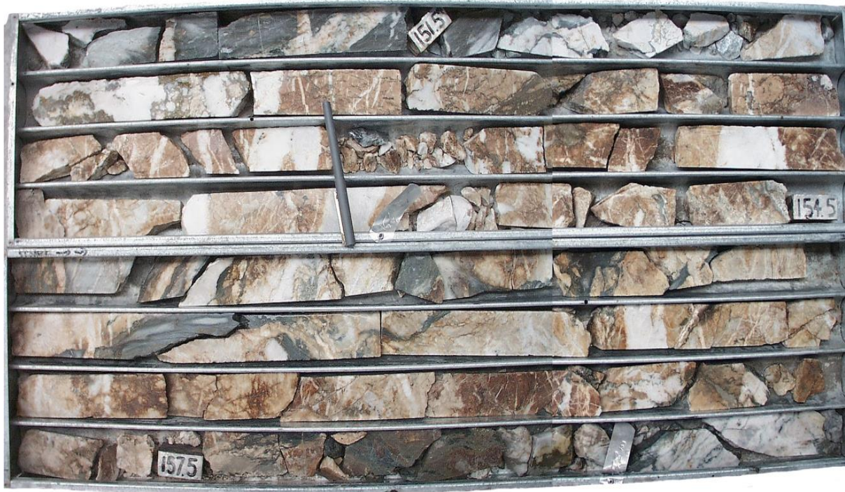
figure 4.4: DDH97BC11 - CRA/Rio Tinto (tray from 151.1m to 158.2m) part of 142m–160m, 18m @ 0.44% Cu showing silica+dolomite alteration with chalcopyrite. Similar style of mineralisation to Mt Isa.
