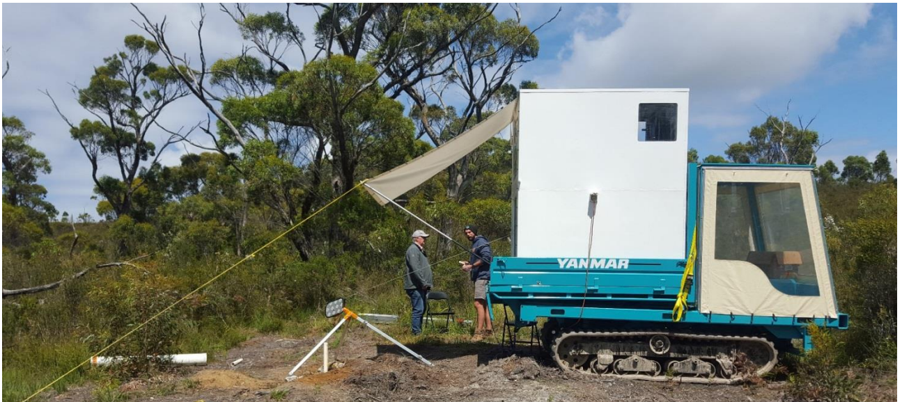
figure 5.2: DigiAtlantis EM system surveying hole at Balfour
