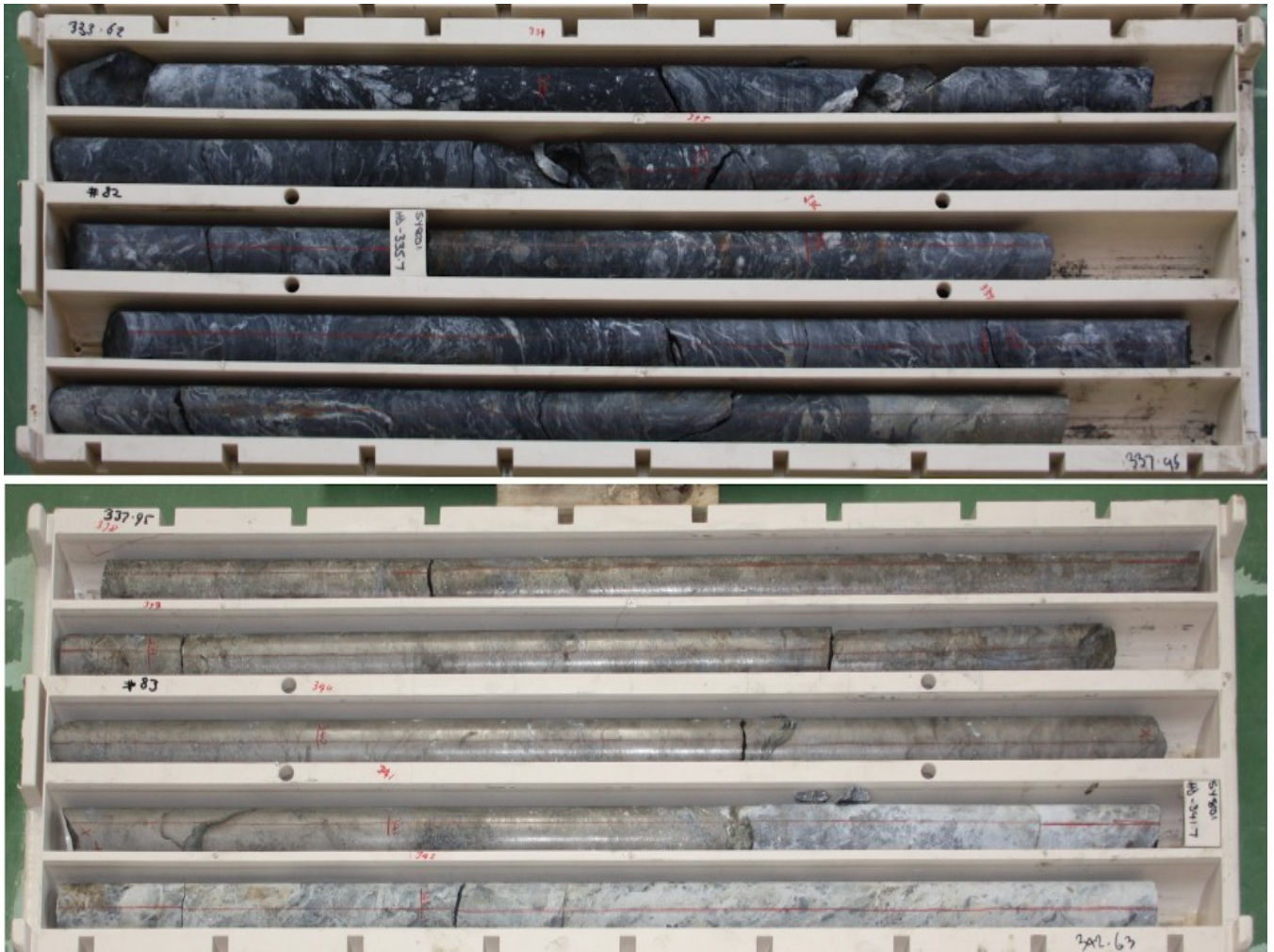
Figure 9: Balstrup Fault mineralisation – transition from siltstone cataclasite to altered dolomite
