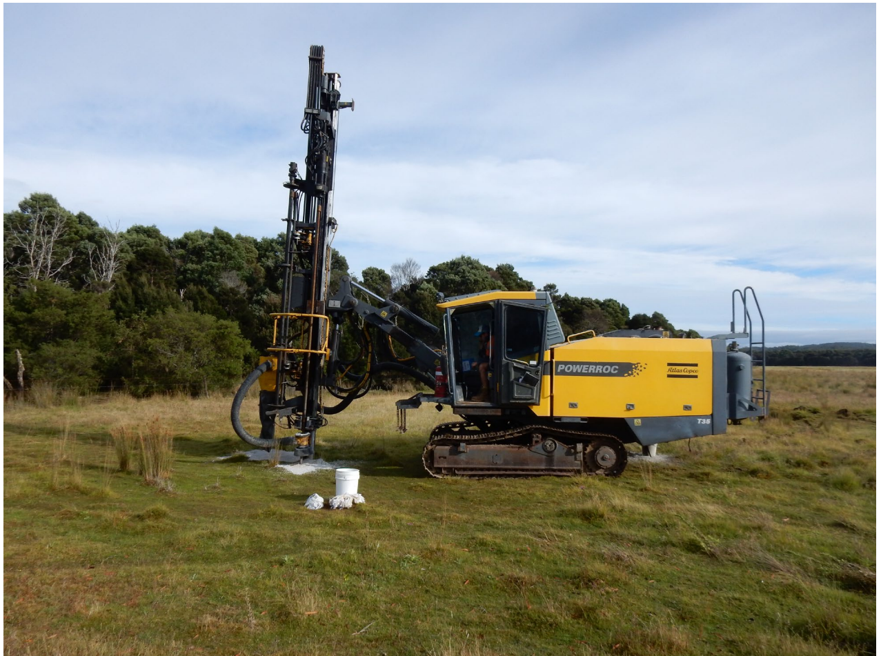
Figure 4. Cresswells Blast Hole Percussion Rig Drilling Donalds Road Dolomite
