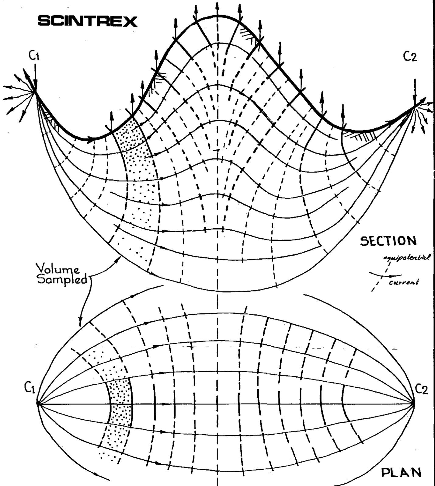
Diagrammatic Representation of Primary Current and Potential Field in Steep Topography.
