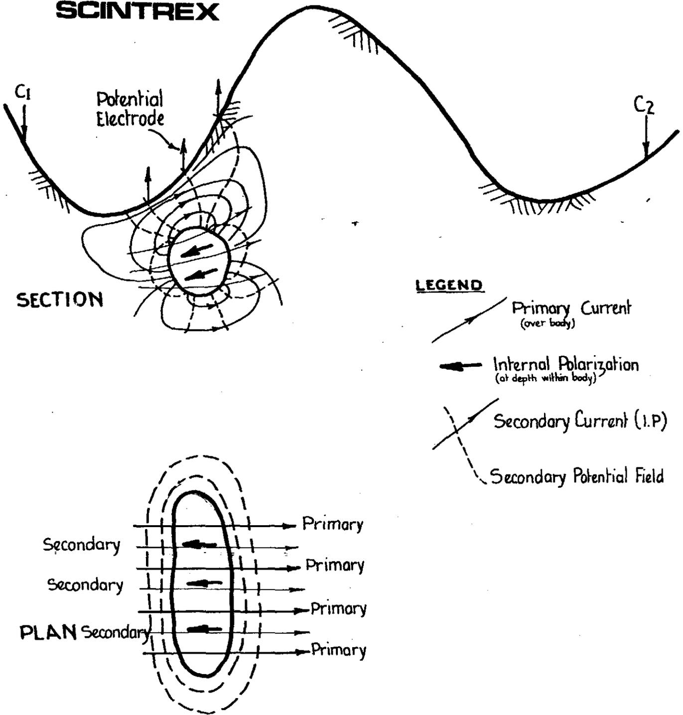
Diagrammatic representation of secondary current (I.P.effect) and secondary potential field in steep terrain.
