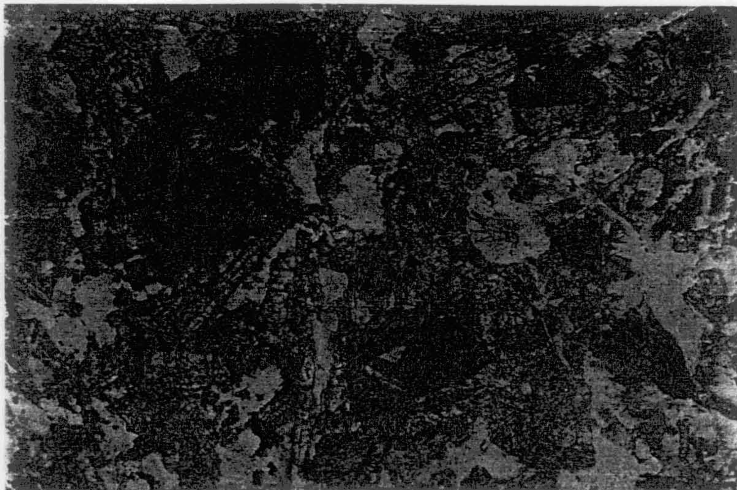
Sample 3757233. Relict igneous brown-green hornblende, altered plagioclase laths in a matrix of chlorite and minor other phases. Plane light. FOV is 2.64 mm.
