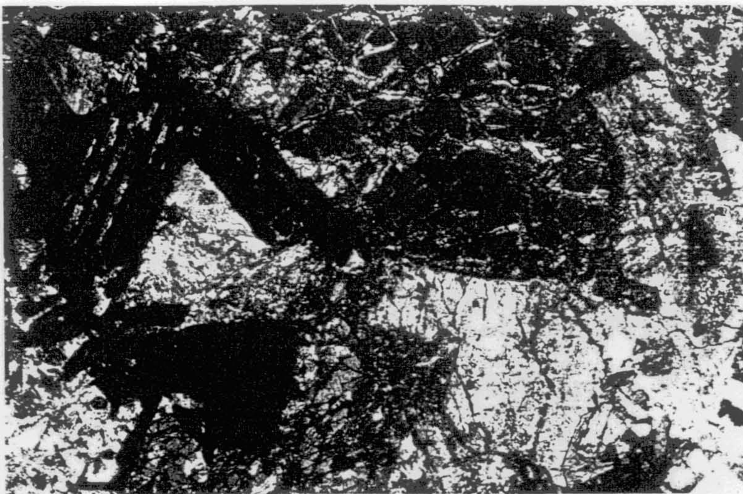
Sample 3757234. Very coarse grained igneous mineralogy with pegmatoidal texture consisting of olivine, plagioclase, highly skeletal ilmenite and minor hornblende. FOV is 2.64 mm.
