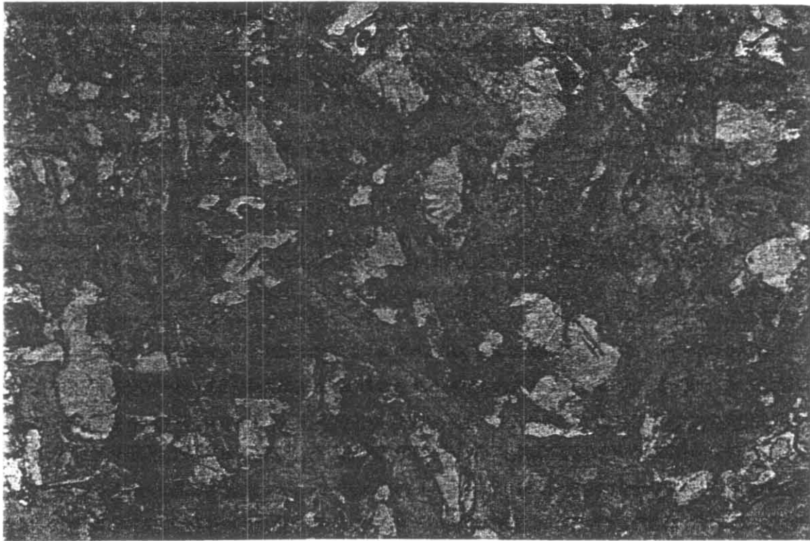
Sample 3911787. Igneous-textured laths, probably of plagioclase, pseudomorphed by very fine-grained chlorite in a matrix of plagioclase and quartz with minor titanite after ilmenite. FOV is 2.64 mm.
